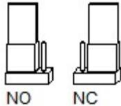
You are able to change the relay function to normally open (NO) or normally closes (NC) using jumper 21 on the circuit board.
