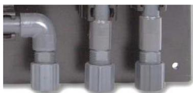
2. Connect the drain reagent with reinforced tube 6x12mm to a drain. Make sure there is enough slope.
